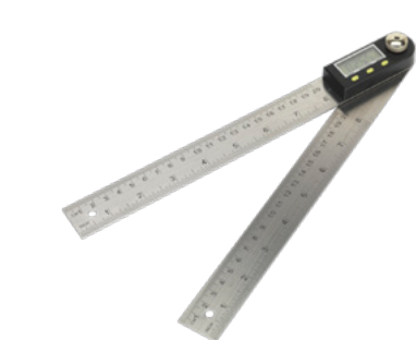
• Indispensable tool ideal for woodworking, construction and machining. • An angle finder that doubles as a rule. • Perfect for finding both internal and external angles. • The digital display is clear with easy calibration. • Measuring range from 0o to 360o. • Metric/Imperial rule which can be locked in any position. • Rule Length: 200mm(8").
