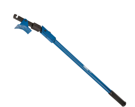
Expert Quality, for tensioning wire (including barbed wire) up to 4mm diameter prior to stapling onto wooden fencing posts. Manufactured from carbon steel hardened and tempered with 600mm long handle for excellent leverage and a pivoting 'Durbar' steel locating foot to grip any post type whilst straining wire. Display packed.
