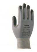
Seamless ultra-soft and flexible glove that stretches effortlessly with the hand. Robust NBR coating still allows a good tactile feel. Ideal for drv and wet applications. Resistant to oil / grease. Good general maintenance, precision, repair glove. EN 388:2016 (4131X). Sizes 7 (S) to 10 (XL)
