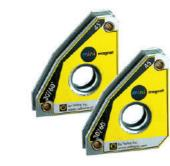
$30^{\circ}\,/\,60^{\circ}$  edge, with the standard 45° and right angles Large centre hole for easier handling Two riveted holes (for 6-32 screws) for linking magenets together Dimensions 59 x 50 x 16mm 10kg Max. Pull
