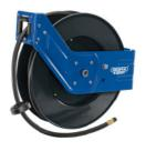
Expert Quality, 3/8" rubber air hose, the latching mechanism provides 20 bar max operating pressure. The airline stops in any position and the reel can be solidly mounted to a ceiling/wall or vehicle. (note: does not have 180anddeg; bracket).|Hose size: 3/8"Hose connection: 1/4 BSP threadMax. working pressure: 20 bar (300psi)Operating temperature: -5 to 45?
