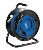
Air hose reel with polyethylene hose fitted with 1/4" BSP brass connectors. 20m of durable hose Maximum working pressure of 20bar. Sturdy hose reel made from steel with floor standing frame and carry handle
