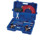
Complete set of regulators and torches for oxyacetylene welding. Includes single stage gas regulators with two gauges to show bottle pressure and working pressure. Two colour coded gas hoses with flashback arrestors and standard 3/8" BSP connectors. Welding torch with three lightweight nozzles. Supplied with sturdy plastic storage case.
